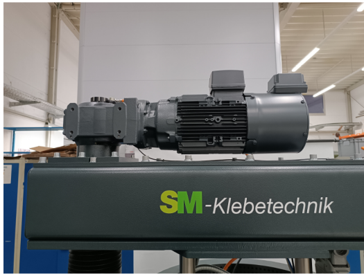
Material conveying without compressed air using an electric spindle drive
