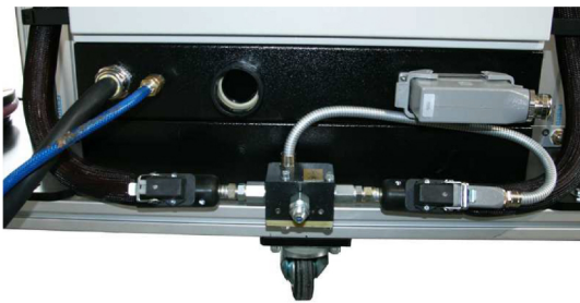
Heated hose changeover manifold with included mechanical check valve to maintain material flow direction
