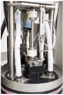
Pneumatic piston driven ball valve for deaeration
