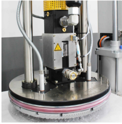
Screw pump and automatic de-aeration module
